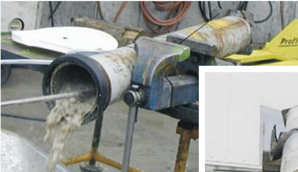
**Tackling the concrete with an extended lance and a rotating nozzle.**
