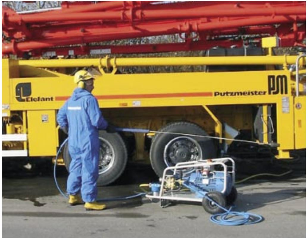
**It doesn't often happen – but it can. The concrete pump is blocked. And rapid, efficient handling is the order of the day. Cleaning the blocked pipe using high-pressure is both an effective and an economically interesting solution.**
