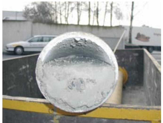
pipes which have been blocked with set concrete for up to 24 hours can be thoroughly cleaned.
