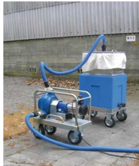
With a pump, the cleaning water can be channelled into the optional filter system, which separates the dirt from the water.
