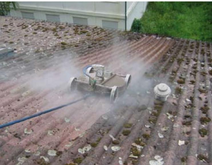
The DRS cleaning system can cover even large roof surfaces thoroughly, quickly and without having to walk on the roof.
