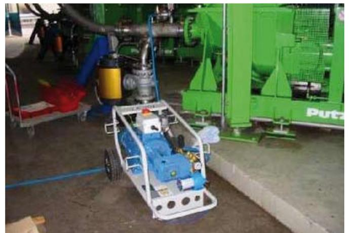
The Dynajet® high-pressure cleaner is ideal for rinsing and unblocking pipelines. (here: Dynajet® 350<sup>m</sup> cleaning a sewage sludge feed pipeline)
