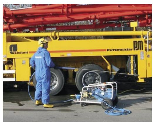
It doesn't often happen – but it can. The concrete pump is blocked. And rapid, efficient handling is the order of the day. Cleaning the blocked pipe using high-pressure is both an effective and an economically interesting solution.
