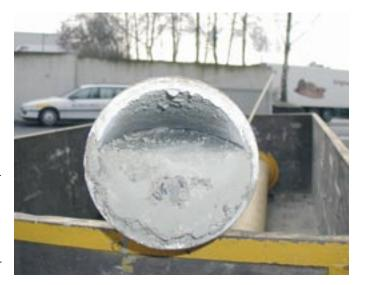
pipes which have been blocked with set concrete for up to 24 hours can be thoroughly cleaned.
