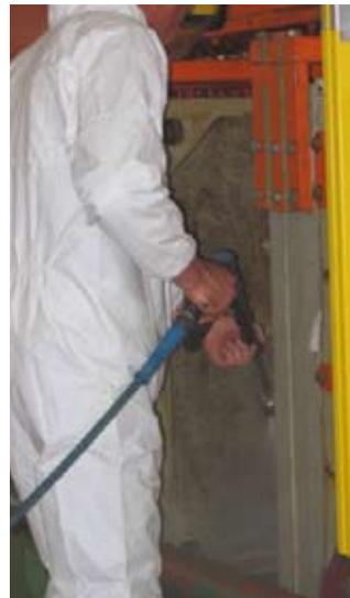
**Filter presses in sewage treatment plants are cleaned quickly and thoroughly with high-pressure. (here: Dynajet® 500<sup>me</sup>)**
