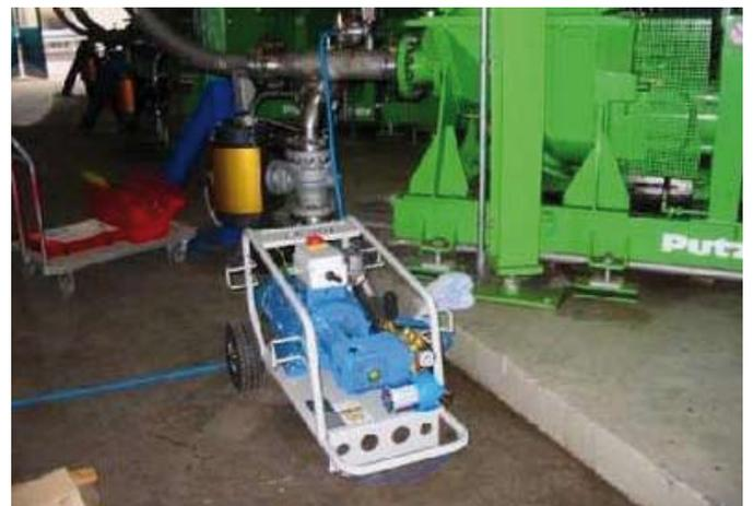
The Dynajet® high-pressure cleaner is ideal for rinsing and unblocking pipelines. (here: Dynajet® 350<sup>me</sup> cleaning a sewage sludge feed pipeline)
