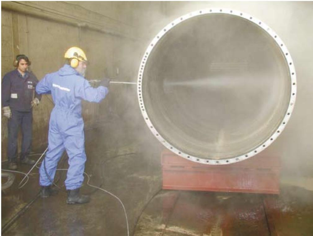
High pressures are necessary for preparing contaminated units prior to daily use. (here: cleaning/ servicing a rotary screen filter)
