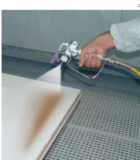
Even enamel can be perfectly processed with Putzmeister airless devices.
