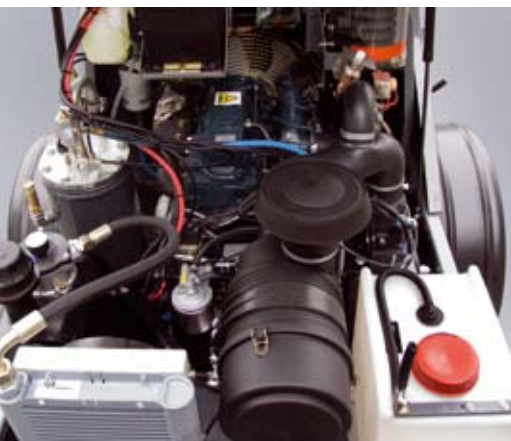
The new water-cooled diesel motor complies with the most recent emission standards (COM III).
