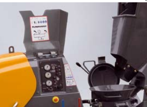
The analogue instruments are easy to read and intuitive to operate. A durable flap protects the instruments reliably against dirt and damage.
