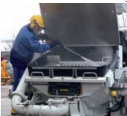
3 With a water pressure of 330 bar you can remove all types of dirt
