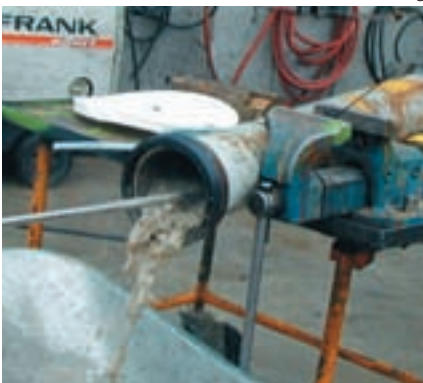
5 Concrete blockages in the delivery line can be removed efficiently with Dynajet® 350 m g Plus
