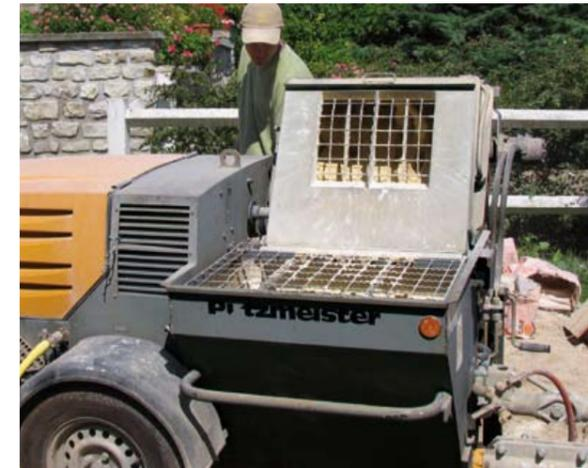
But it gets even better. BMR models have a lifting mixer, on which a powerful hydraulic system does all the work.
