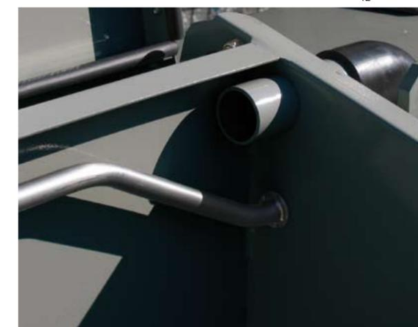
The optional dust extraction is integrated in the mixer grid (SP 11<sup>SM</sup>).
