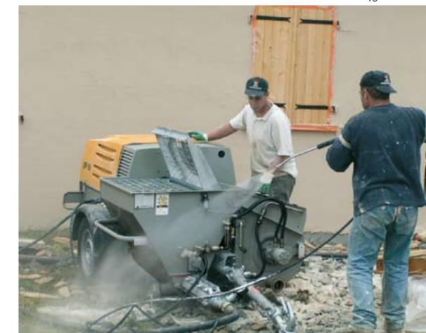
Once your work is finished, you can clean your Beliso with the integrated 120 bar high-pressure cleaner – quickly and efficient.
