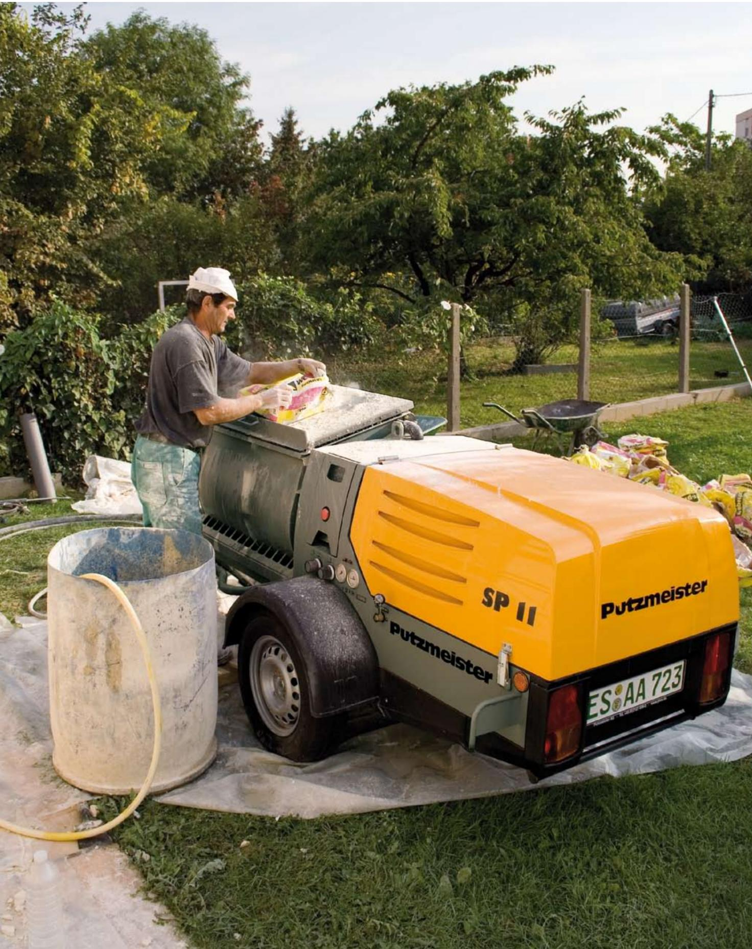
The **trap mixer** (SP 11<sup>BMT</sup>) is the simple, robust and cost-effective variant. This mixer is fixed to the machine. The prepared material flows through a flap in the bottom of the mixer into the hopper of the SP 11.
