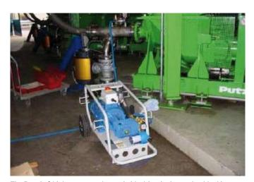
The Dynajet® high-pressure cleaner is ideal for rinsing and unblocking pipelines. (here: Dynajet® 350 ™ cleaning a sewage sludge feed pipeline)
