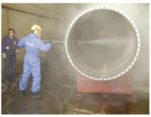
High pressures are necessary for preparing contaminated units prior to daily use. (here: cleaning/ servicing a rotary screen filter)
