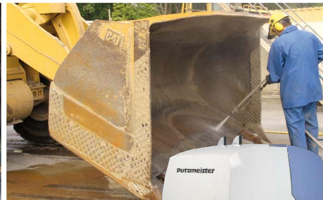
High demands in industrial cleaning and construction industry require a **Dynajet® hot water** solution with 800 bar (11,600 PSI). The Dynajet® 800<sup>th</sup> is one of the worldwide few high-pressure jetting systems with hot water up to 800 bar (11,600 PSI).
