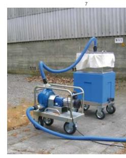
With a pump, the cleaning water can be channelled into the optional filter system, which separates the dirt from the water.
