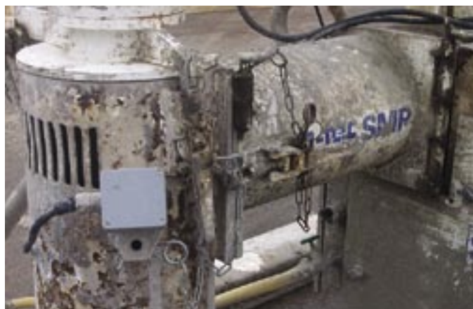
Even these hardened concrete residues had no chance against the power of the Dynajet 350 th
