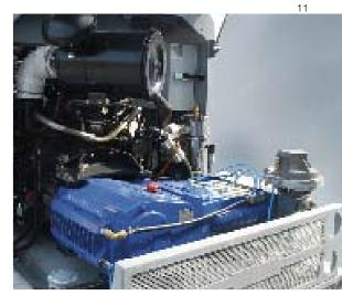
The horizontal design of the robust triplex-plunger high-pressure pump saves space and quaranties, easy service and maintenance work.
