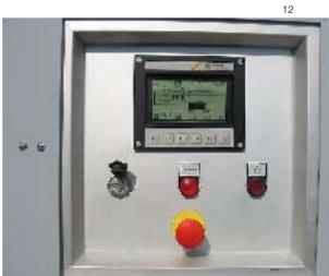
Easy control system with convenient automatic pressure/ speed control (manual operation is optional).
