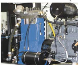
The high-pressure pump is installed in an upright position, thus saving considerable space.
