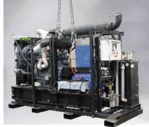
The installation version of the maximum-pressure unit Dynajet UHP 250 (without soundproofing cover is mounted on a support frame).
