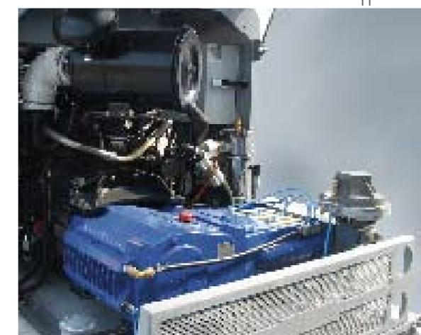
The horizontal design of the robust triplex-plunger high-pressure pump saves space and quaranties, easy service and maintenance work.
