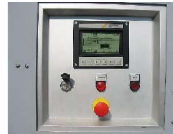
Easy control system with convenient automatic pressure/speed control (manual operation is optional).
